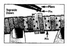
With long-nose pliers or tweezers, carefully pull out connecting U-shaped pins between adjacent links on the top side and the underside.
