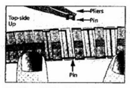
5. When the band is ready to be reassembled, place both sides together in front of you, top-side up. With long-nose pliers or tweezers, reinsert the U-shaped pins in the top and underside of the connecting band links. Bend the side wing back down on the top link and underside link.
